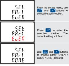
On completion of the entry procedure, press confirm the setting and press  $^{\text{MA}}$  to return to the main
