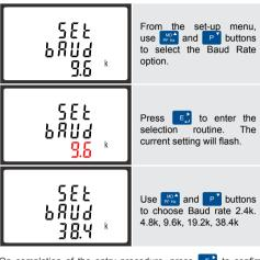
On completion of the entry procedure, press [ to confirm the setting and press MA to return to the main set up menu.
