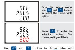
On completion of the entry procedure press [] to confirm the setting and press MA to return to the main set up menu.
