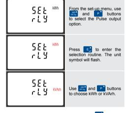
On completion of the entry procedure, press [1] to confirm the setting and press MA to return to the main set up menu.
