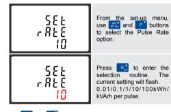
Use public and buttons to choose pulse rate. On completion of the entry procedure, press [ to confirm the setting and press [V/A] to return to the main set up menu.
